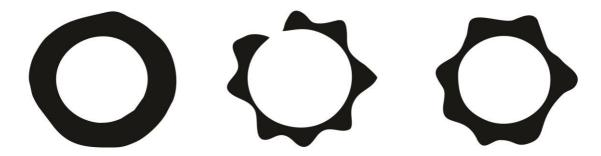
Figure 3.3 Real fabric drape images obtained from the physical experiments (drapemeter)
