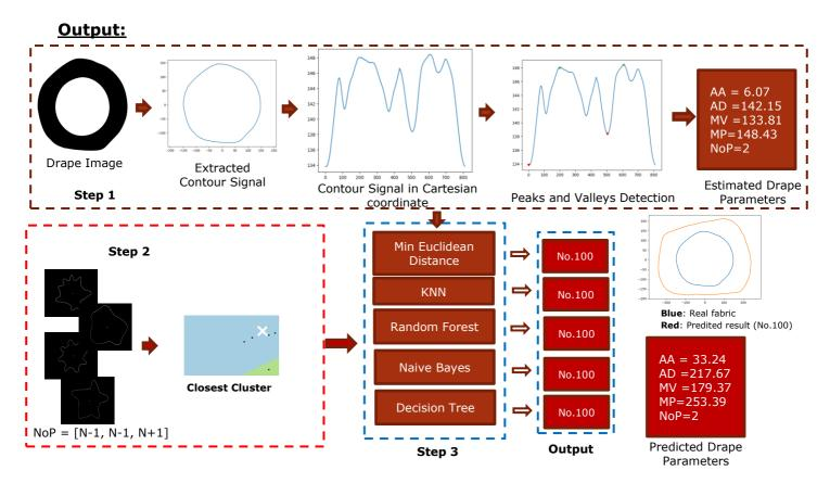
Figure 3.5 Testing in a real fabric (Drape example)
